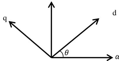
Figure 2. Relationship between  $\alpha - \beta$  and d-q coordinate system
