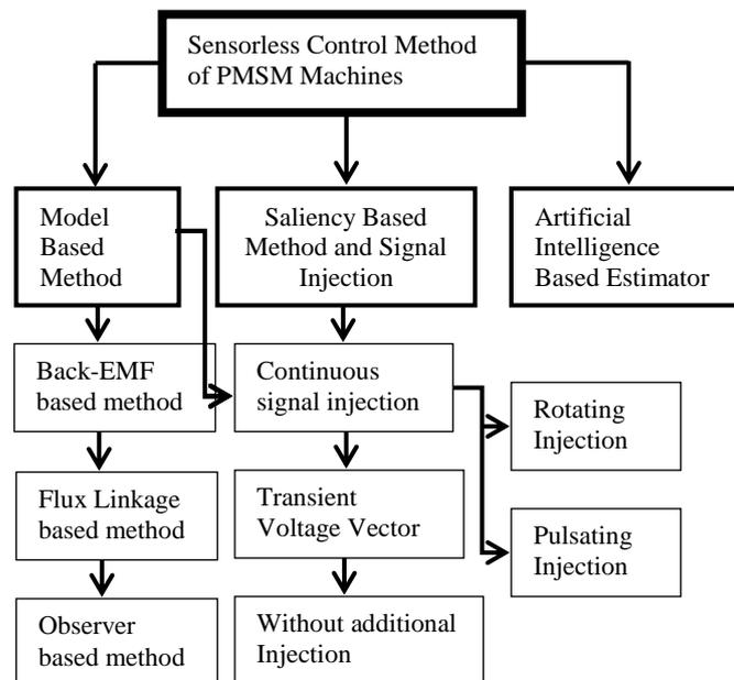
Figure 1. Classification of sensorless control method of PMSM
